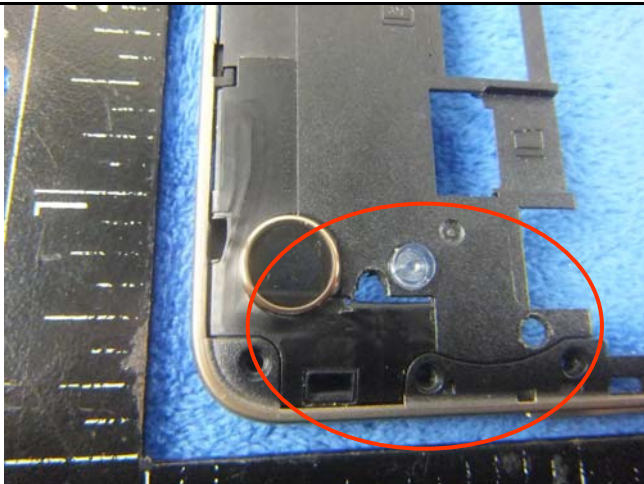
LTE - Antenna View
