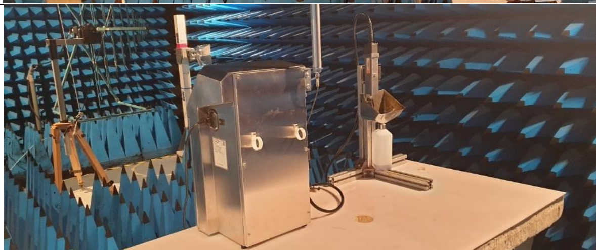
Test setup in anechoic chamber – Frequency <1GHz
