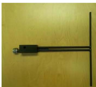
Figure 1 – MVG COMOSAR Validation Dipole
