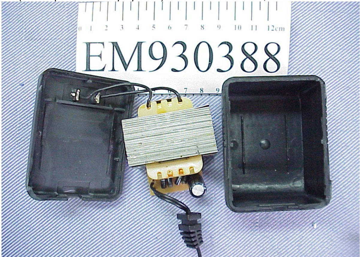
Photos 56 (AC Adapter for Desktop Speaker) Transformer & PCB View
