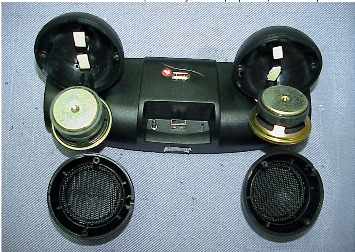
Photos 54 (Accessory, Desktop Speaker) Internal Speakers View
