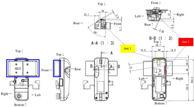
\*When the SAR test was performed, the part of Blue enclosing line was removed.
