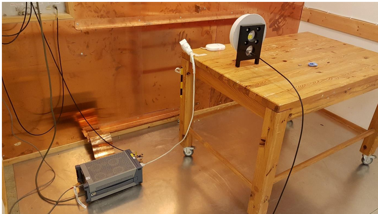
Photo of the test setup for conducted emission
