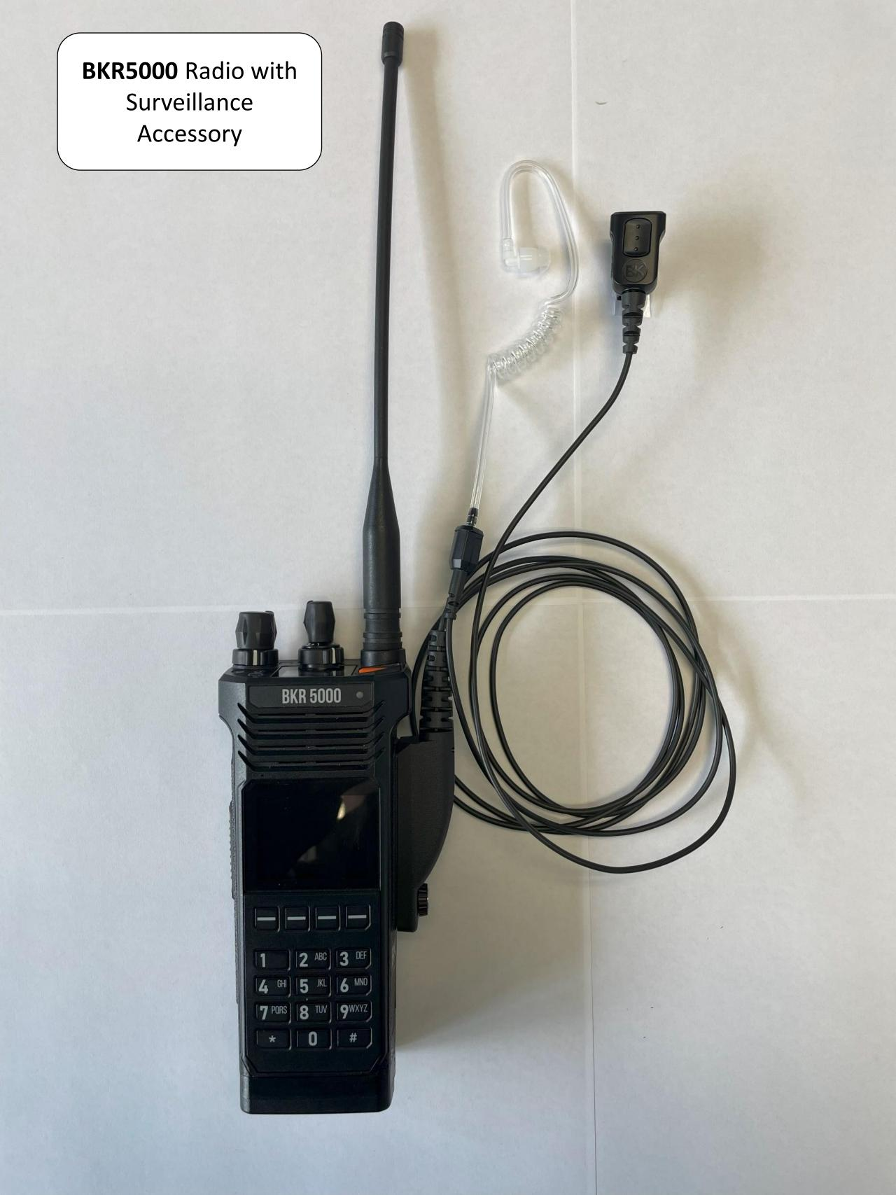
**BKR5000** Radio with Nylon Holster (BKR0415B) and BKRangeMax<sup>™</sup> Antenna (BKR0813)
