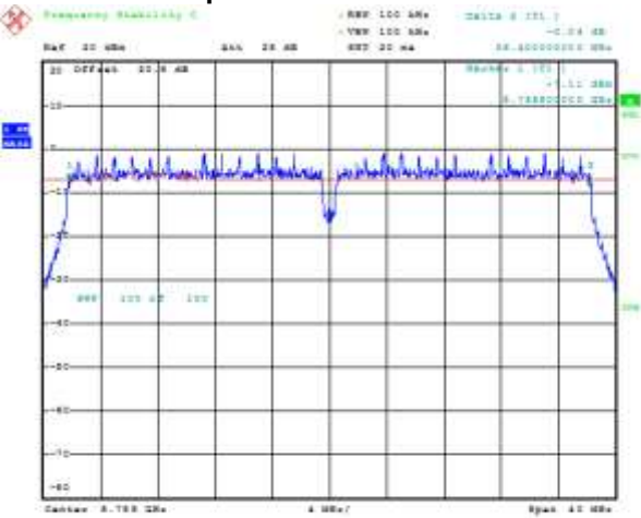
Figure 8-20: 6 dB Bandwidth Secondary, 802.11ac, Channel 149, MCS0 Mbps
