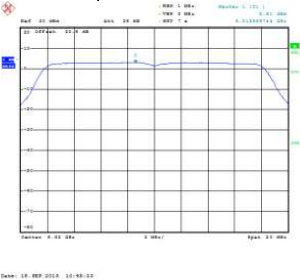
Figure 7-68: Peak Power Spectral Density SISO Primary, 802.11a, Channel 64, 6 Mbps
