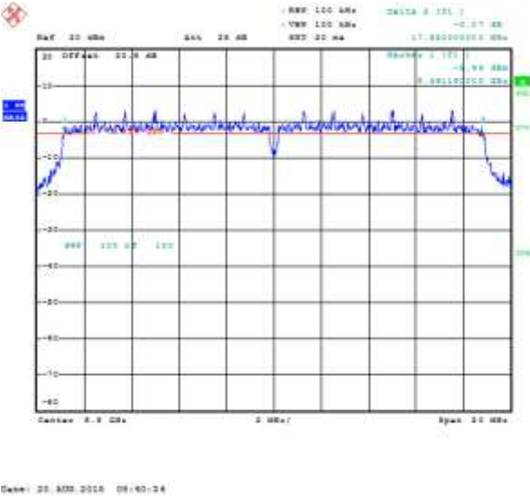
Figure 7-15: 6 dB Bandwidth Primary, 802.11n, Channel 100, MCS 0
