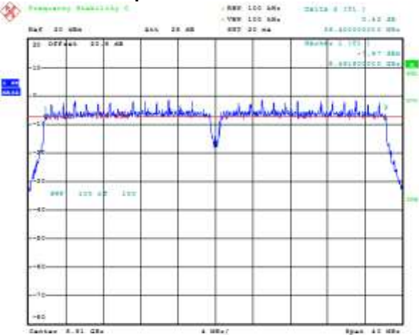
Figure 8-18: 6 dB Bandwidth Secondary, 802.11ac, Channel 100, 6 Mbps
