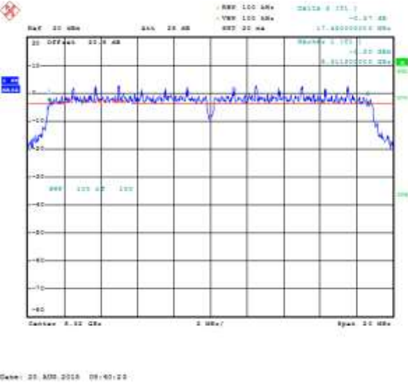
Figure 7-14: 6 dB Bandwidth Primary, 802.11n, Channel 64, MCS 0
