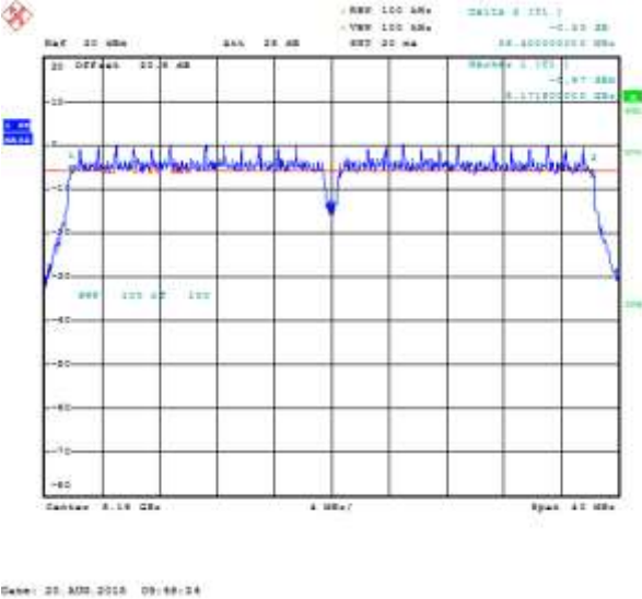
Figure 7-28: 6 dB Bandwidth Secondary, 802.11n, Channel 36, MCS 0
