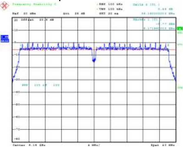
Figure 8-16: 6 dB Bandwidth Secondary, 802.11ac, Channel 36, MCS0 Mbps
