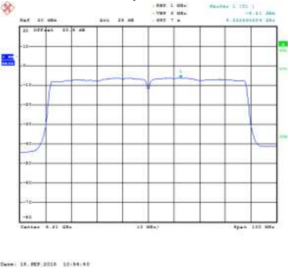
Figure 8-95: Peak Power Spectral Density SISO Primary, 802.11ac, Channel 42, MCS0 Mbps
