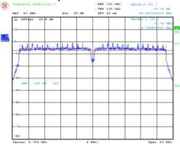
Figure 8-15: 6 dB Bandwidth Primary, 802.11ac, Channel 149, MCS0 Mbps
