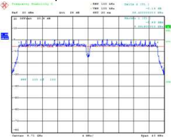
Figure 8-19: 6 dB Bandwidth Secondary, 802.11ac, Channel 140, MCS0 Mbps
