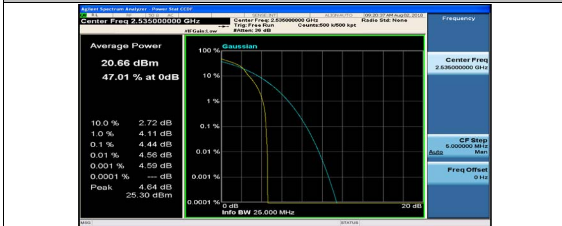
(Channel Bandwidth:20 MHz)_MCH_16QAM_1RB#99
