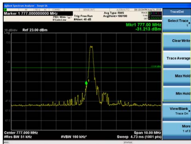
LTE Band 13 QPSK 5MHz CH-Low, 100%RB
