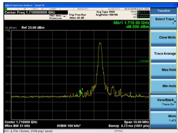
LTE Band 4 16QAM 20MHz CH-High, 100%RB
