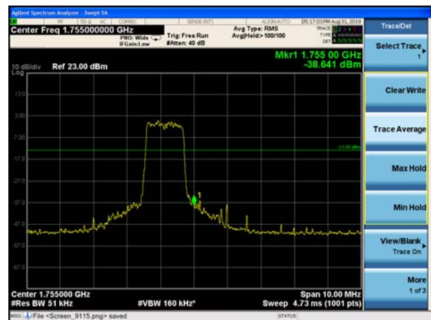
LTE Band 4 QPSK 5MHz CH-High, 1 RB
