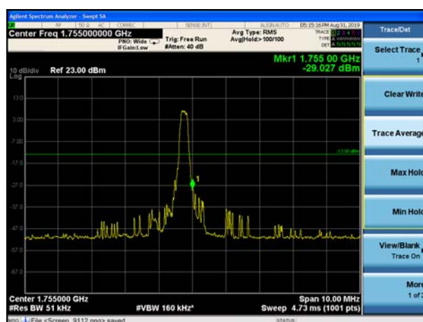
LTE Band 4 16QAM 1.4MHz CH-High, 100%RB
