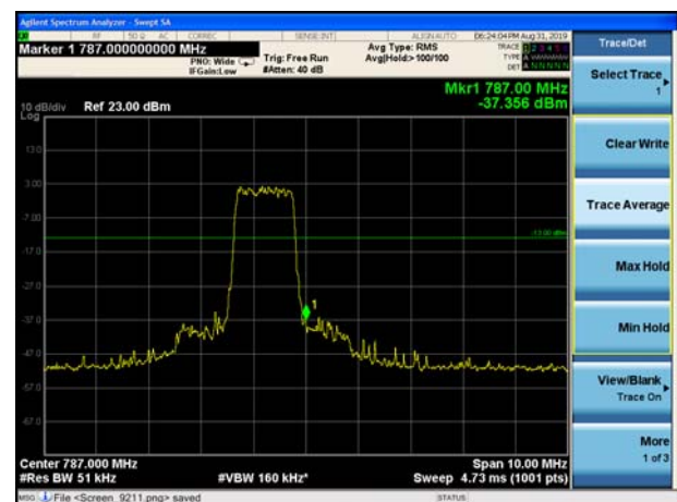
LTE Band 13 QPSK 5MHz CH- High, 100%RB
