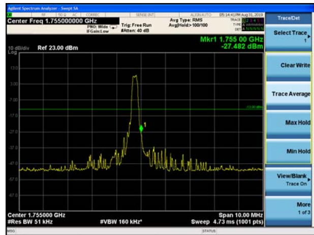
LTE Band 4 QPSK 1.4MHz CH-High, 100%RB
