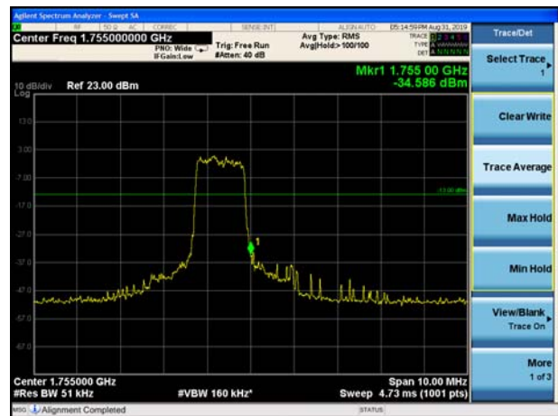
LTE Band 4 QPSK 3MHz CH-High, 1 RB
