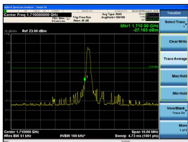
LTE Band 4 16QAM 1.4MHz CH-Low, 100%RB
