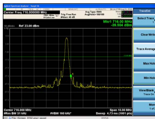
LTE Band 12 16QAM 5MHz CH-High, 100%RB
