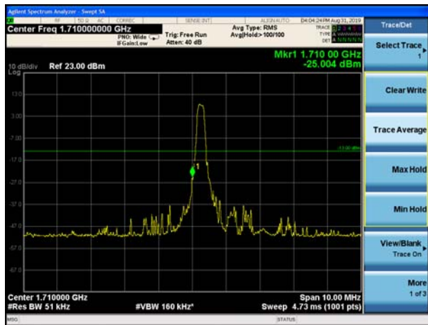
LTE Band 4 QPSK 1.4MHz CH-Low, 100%RB
