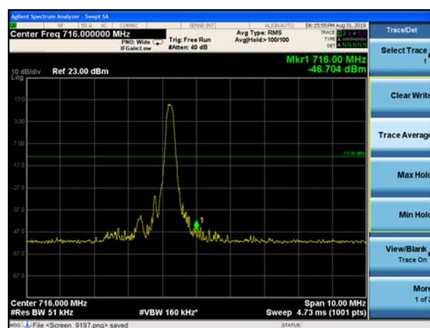
LTE Band 12 16QAM 10MHz CH-High, 1 RB
