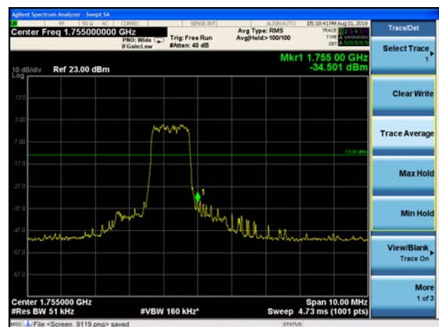
LTE Band 4 QPSK 5MHz CH-High, 100%RB
