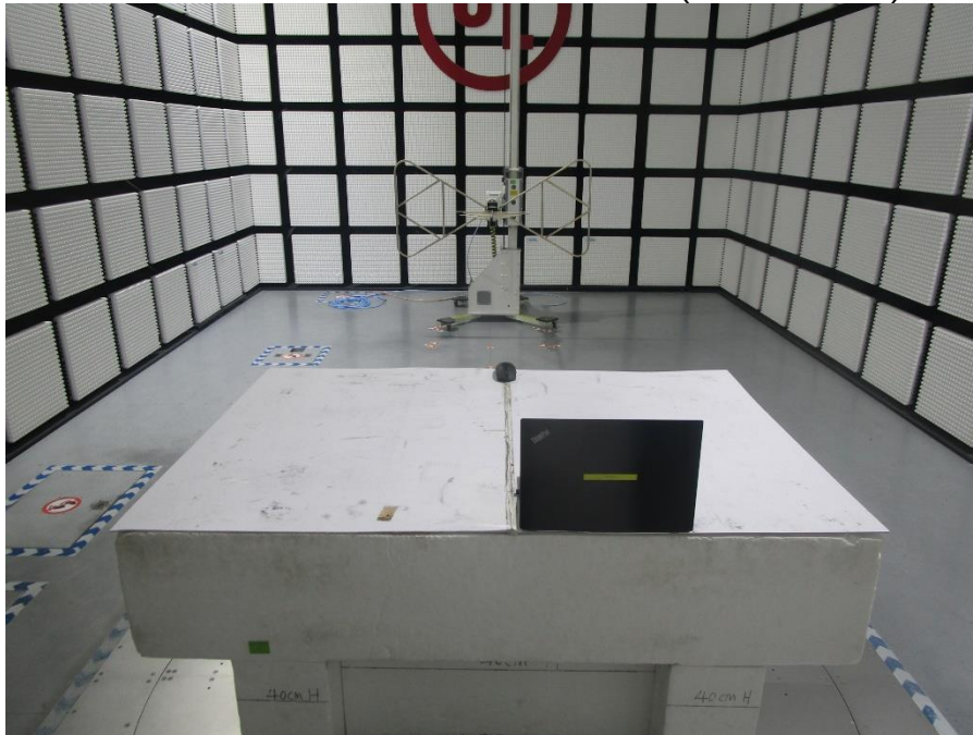
RADIATED RF MEASUREMENT SETUP (Below 30MHz)
