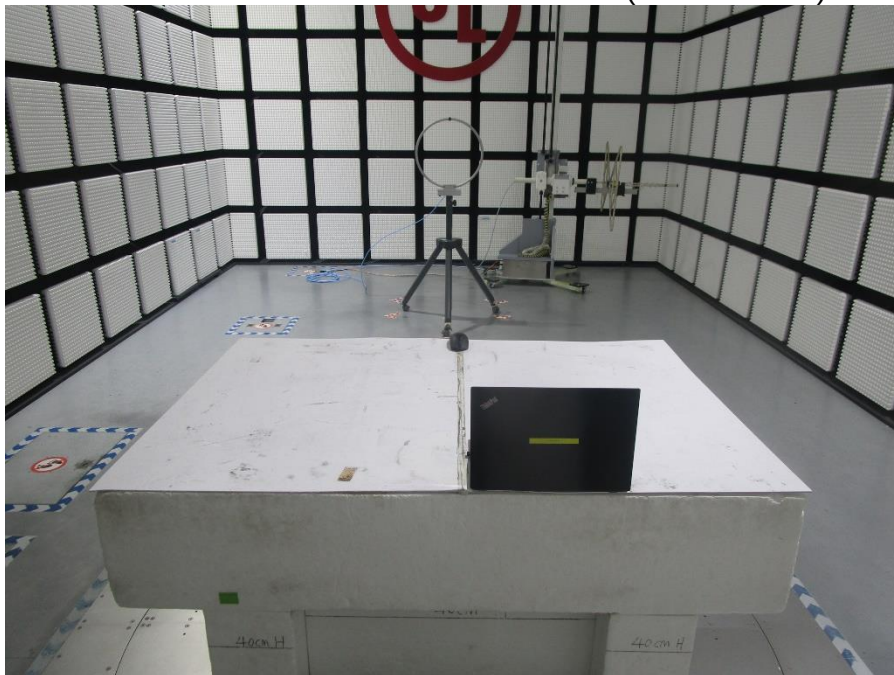
RADIATED RF MEASUREMENT SETUP (Below 30MHz)
