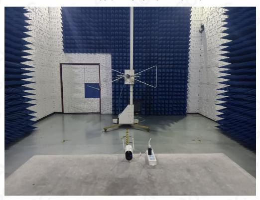
RADIATED EMISSION TEST SETUP ABOVE 1GHz
