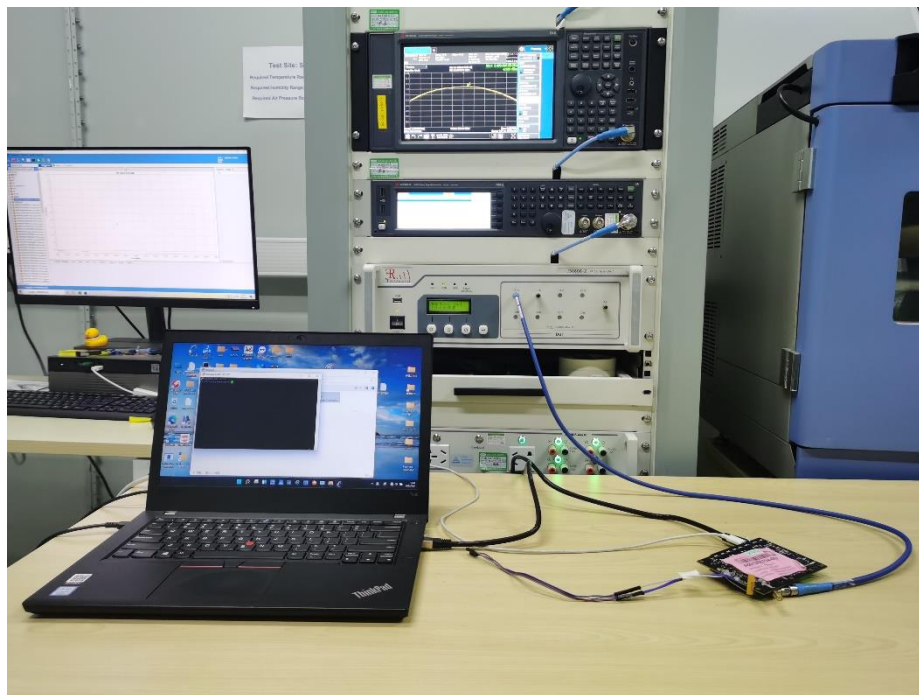
Photograph 3: Set-up photo for RF Conducted Singal test
