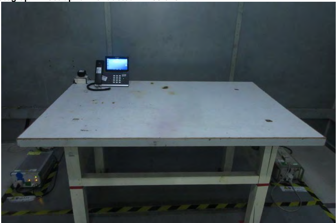
Photograph 4: Set-up for Conducted Emissions
