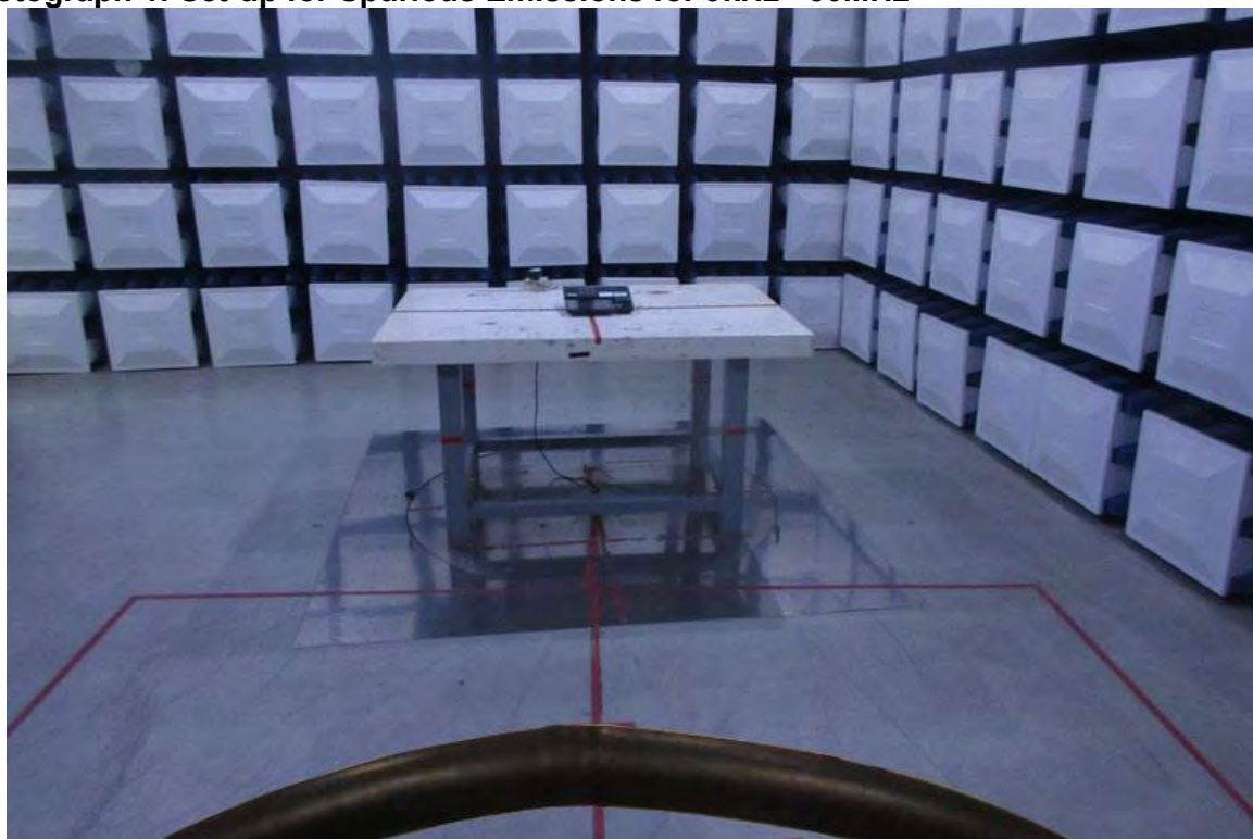
Photograph 2: Set-up for Spurious Emissions for 30 - 1000MHz
