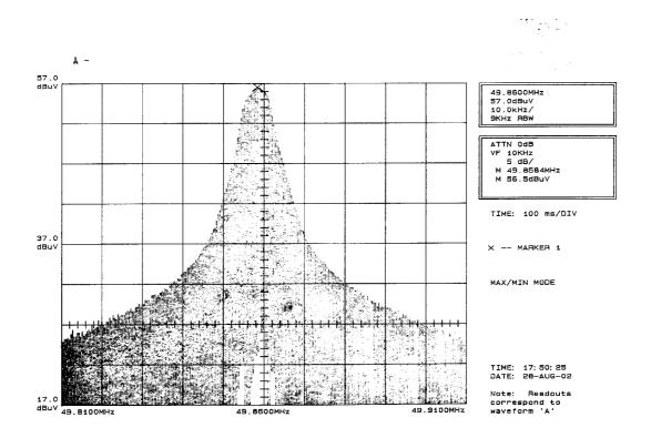
Result : The field strength of any emission within the operation band did not exceed 80 dB( $\mu$ V/m) for average value or 100 dB( $\mu$ V/m) for peak value. Refer to page 9 for the recorded value for the emission at the fundamental frequency.
