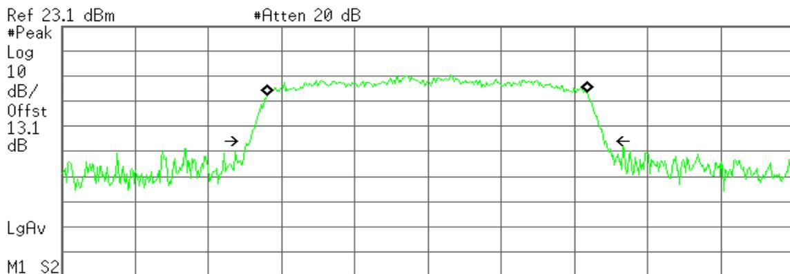
Center 5.180 00 GHz Span 40 MHz
