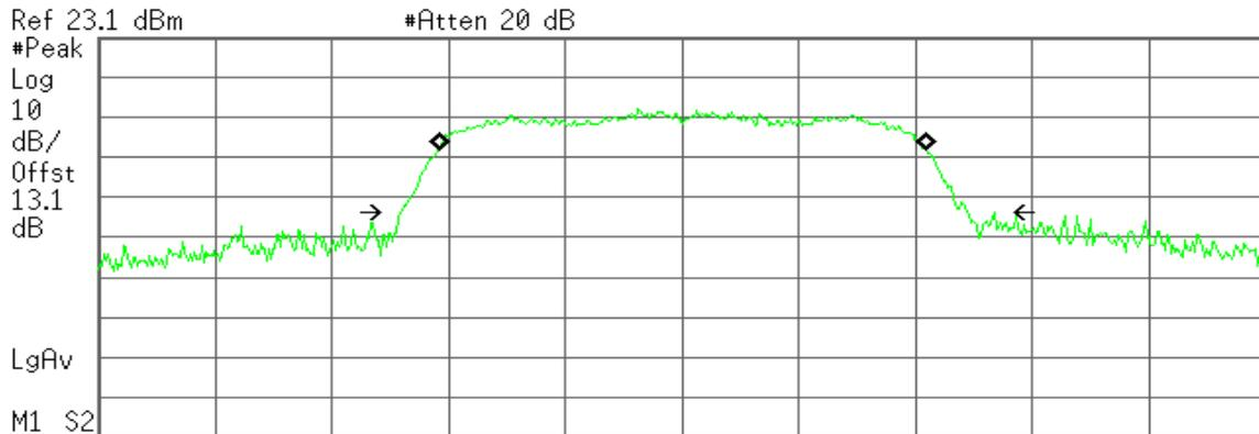
Center 5.260 00 GHz Span 40 MHz
