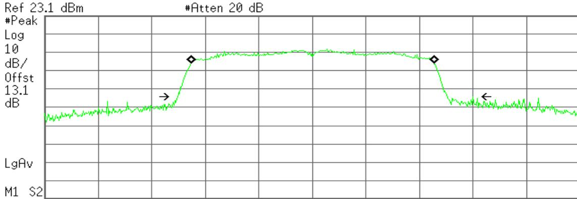
Center 5.510 00 GHz Span 80 MHz
