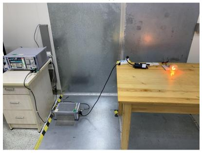
Radiated Spurious Emissions From 30MHz-1000MHz
