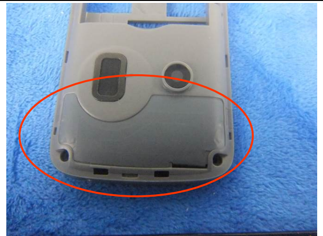
GSM/PCS/UMTS-FDD Antenna View
