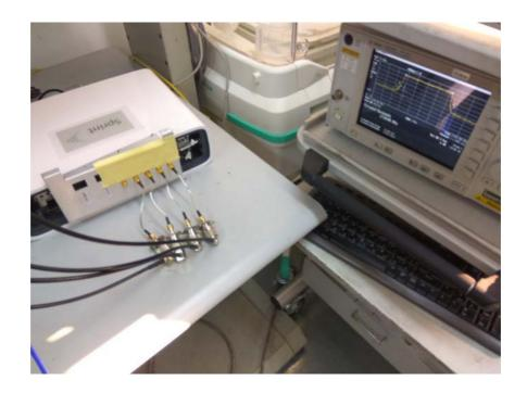
Photograph No.2 Conducted spurious emissions, band edge measurement setup
