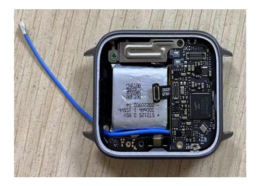
Figure antenna structure
