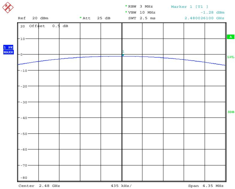
*EDR Mode ( $\pi/4$ -DQPSK)***Low Channel**
