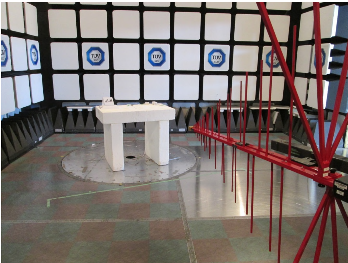
Test setup photo 2 Radiated measurements, 30 MHz – 1 GHz
