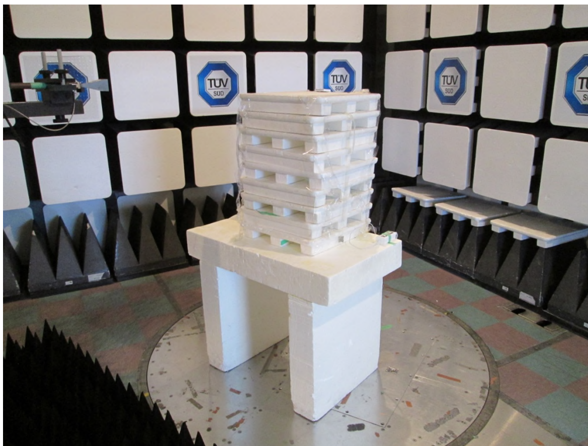
Test setup photo 6 Radiated measurements, 18 GHz – 26.5 GHz
