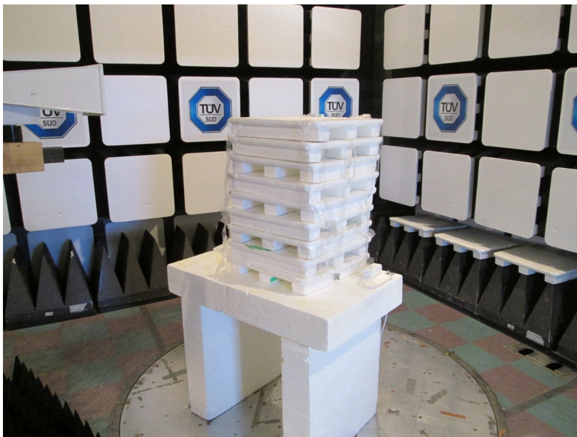
Test setup photo 5 Radiated measurements, 10 GHz – 18 GHz
