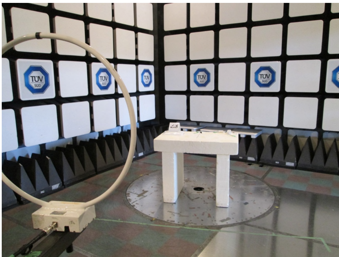
Test setup photo 1 Radiated measurements, 9 kHz – 30 MHz
