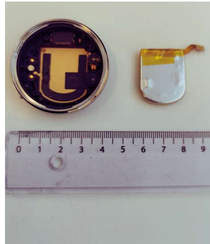
Battery removed bottom
