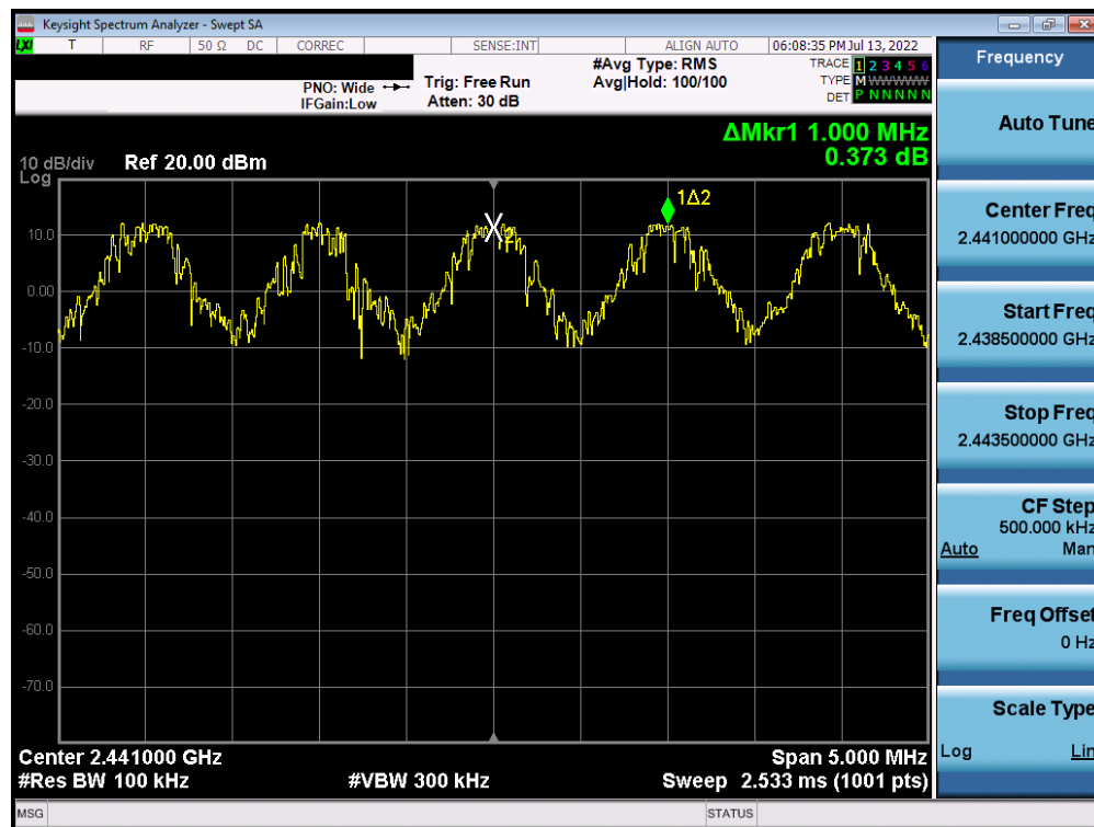
Plot 7-64. Channel Spacing Plot (Bluetooth) – ANT 2
