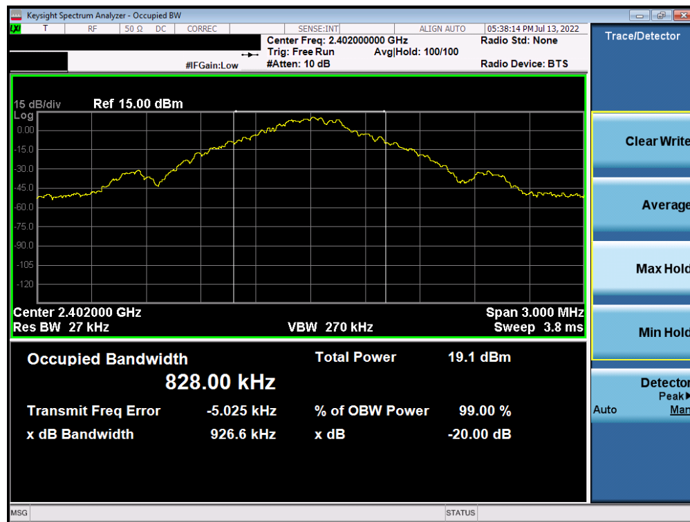
Plot 7-10. 20dB Bandwidth Plot (Bluetooth, 1Mbps – Ch. 0) – ANT 2
