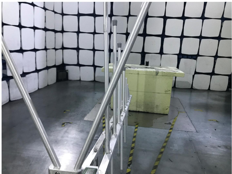
Radiation Emission Test Setup (30MHz to 1GHz)
