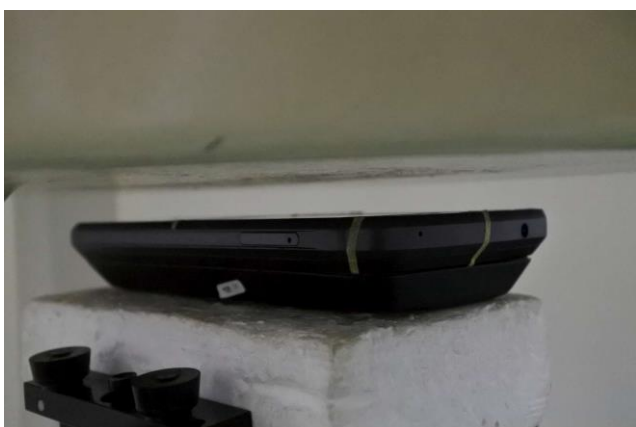
Front With Battery Pack, Test Separation 10 mm
