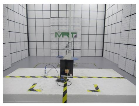
Description: Transmitter Spurious Emissions Test Setup for below 1GHz
