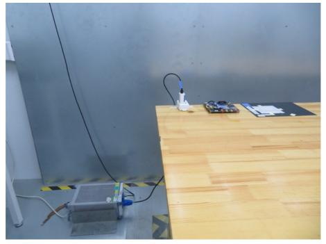
Test Mode: Mode 1 Description: Back View Conducted Emission Test Setup for Power Port
