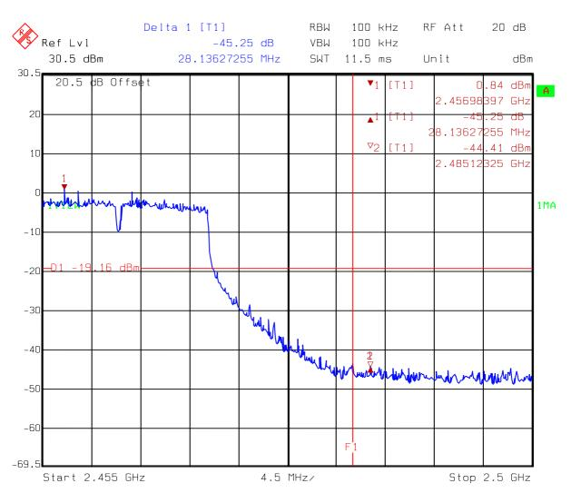
Comment A: Band-edge test at high channel (PK detector)
