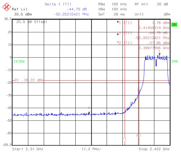
Comment A: Band-edge test at low channel (PK detector)  $802.11g\ F1{=}2390 \text{MHz}$   $F2{=}2400 \text{MHz}$
