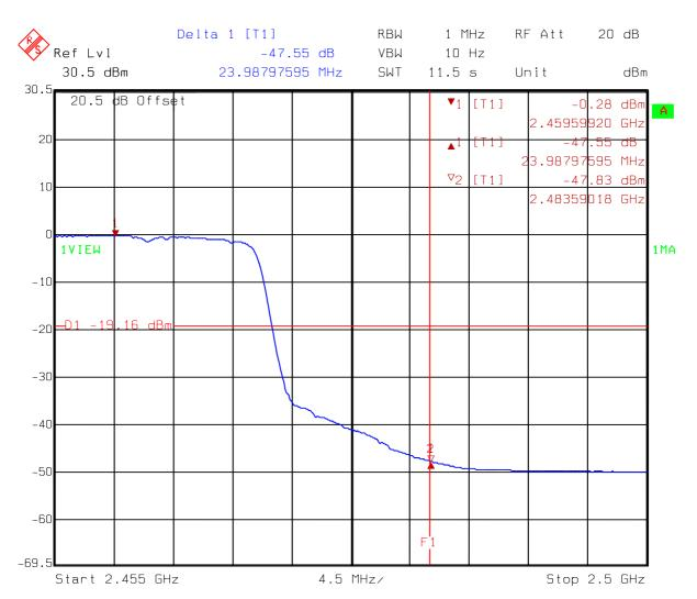
Comment A: Band-edge test at high channel (AV detector)
