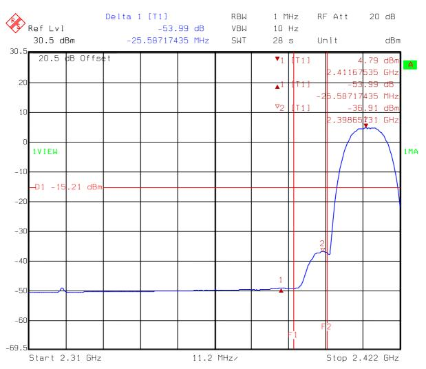
Comment A: Band-edge test at low channel (AV detector)
