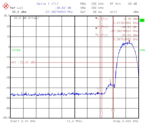
Comment A: Band-edge test at low channel (PK detector)
