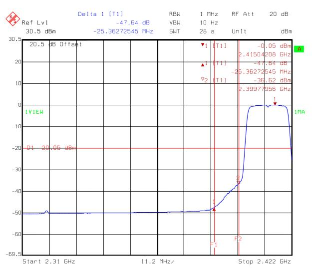
Comment A: Band-edge test at low channel (AV detector)  $802.11g\ F1{=}2390 \rm MHz\ F2{=}2400 \rm MHz$
