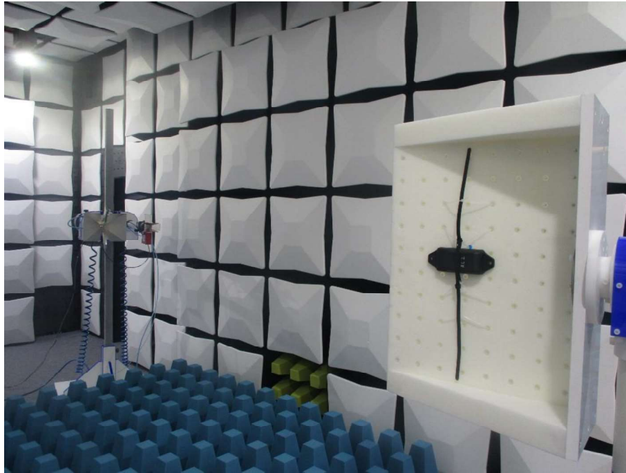
Test Setup: Radiated Measurements (1 GHz to 10 GHz)
