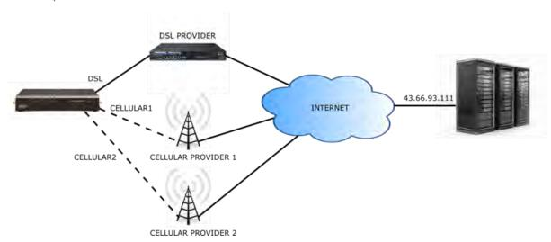
IP probing is configured over the DSL interface. A probe packet of size **256** bytes is sent every **10** seconds to the IP host **43.66.93.111**. If no responses are received for **60** seconds, the TransPort LR device brings the DSL interface down and starts using the **wan2** (**cellular1**) interface.
