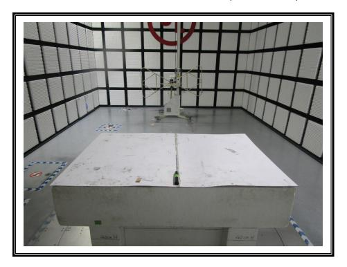
RADIATED RF MEASUREMENT SETUP (Below 30MHz)
