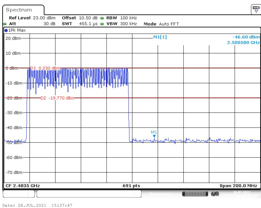
**EDR ( $\pi/4$ -DQPSK): Band Edge-Left Side****Single**
