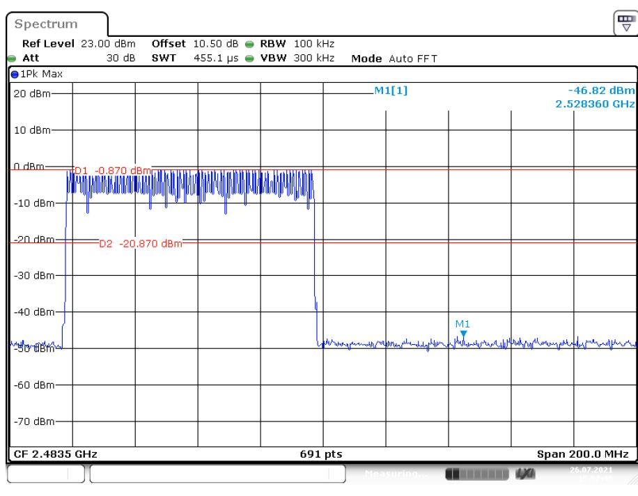
**EDR (8DPSK): Band Edge-Left Side****Single**
