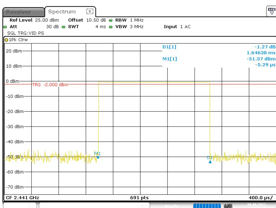
**Pulse time, DH5**
