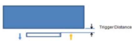
Picture : Proximity sensor triggering distances assessment(Back/front side)
