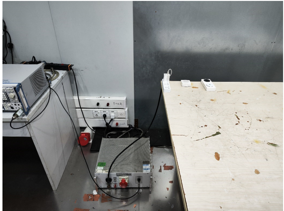
Conducted Emission Test Setup
