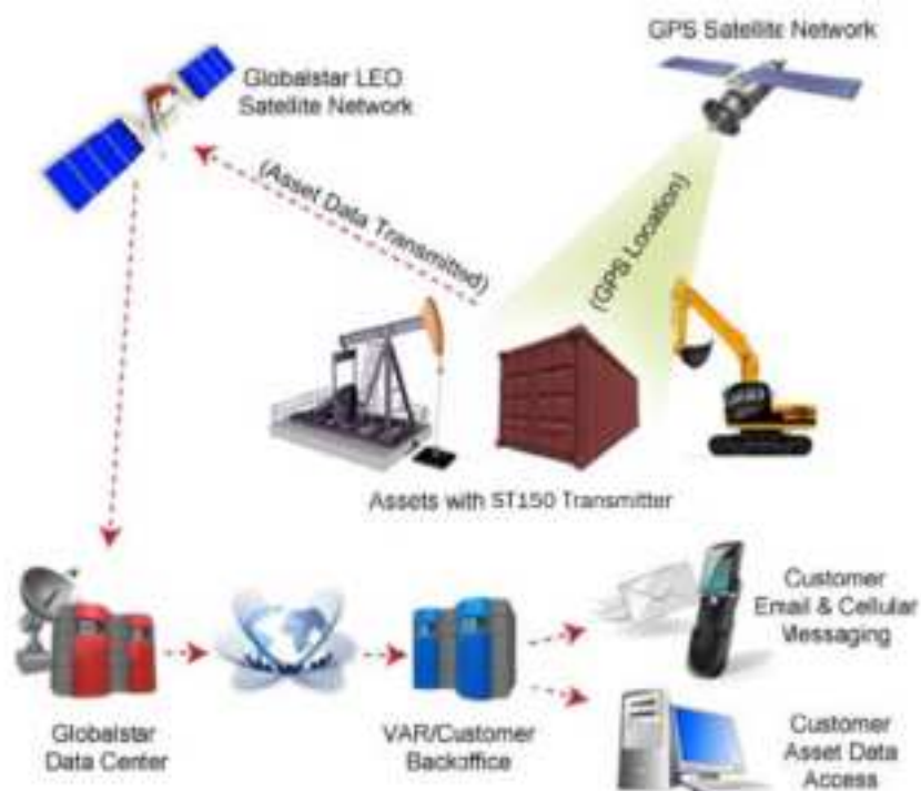
FIGURE 3 - SIMPLEX IOT MESSAGING Data Flow
