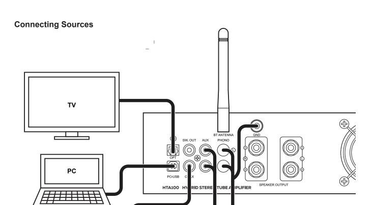
The HTA100 is capable of receiving signals directly from a wide variety of sources. Using high quality cables will ensure the best possible transmission from your connected devices.
