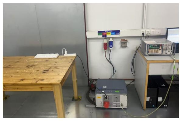
RF CONDUCTED TEST SETUP-FOR BLE
