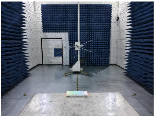
RADIATED EMISSION TEST SETUP ABOVE 1GHz
