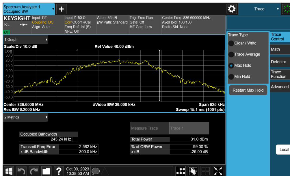
Plot 7-25. Occupied Bandwidth Plot (EDGE, Ch. 190 – Ant E)
