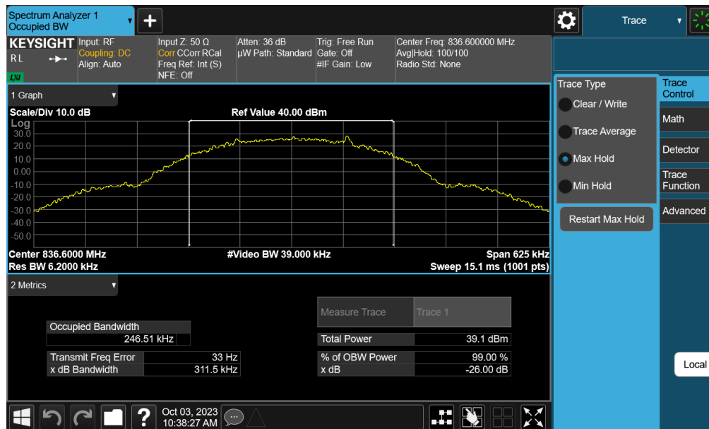
Plot 7-24. Occupied Bandwidth Plot (GPRS, Ch. 190 – Ant E)
