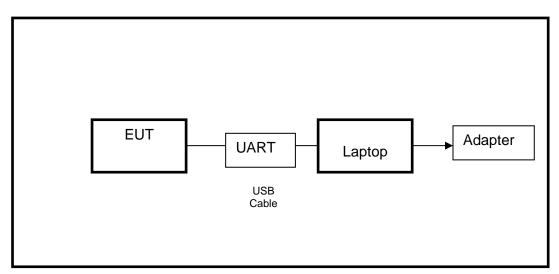
Note: AC adapter only use for AC POWER LINE CONDUCTED EMISSIONS testing.
