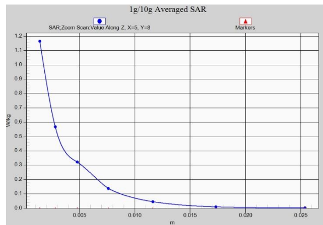
Fig. 1-22 Z-Scan at power reference point (wifi5G)
