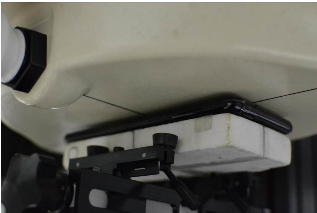
SAR Test Setup Photo 10 – Front Side at 4 mm
