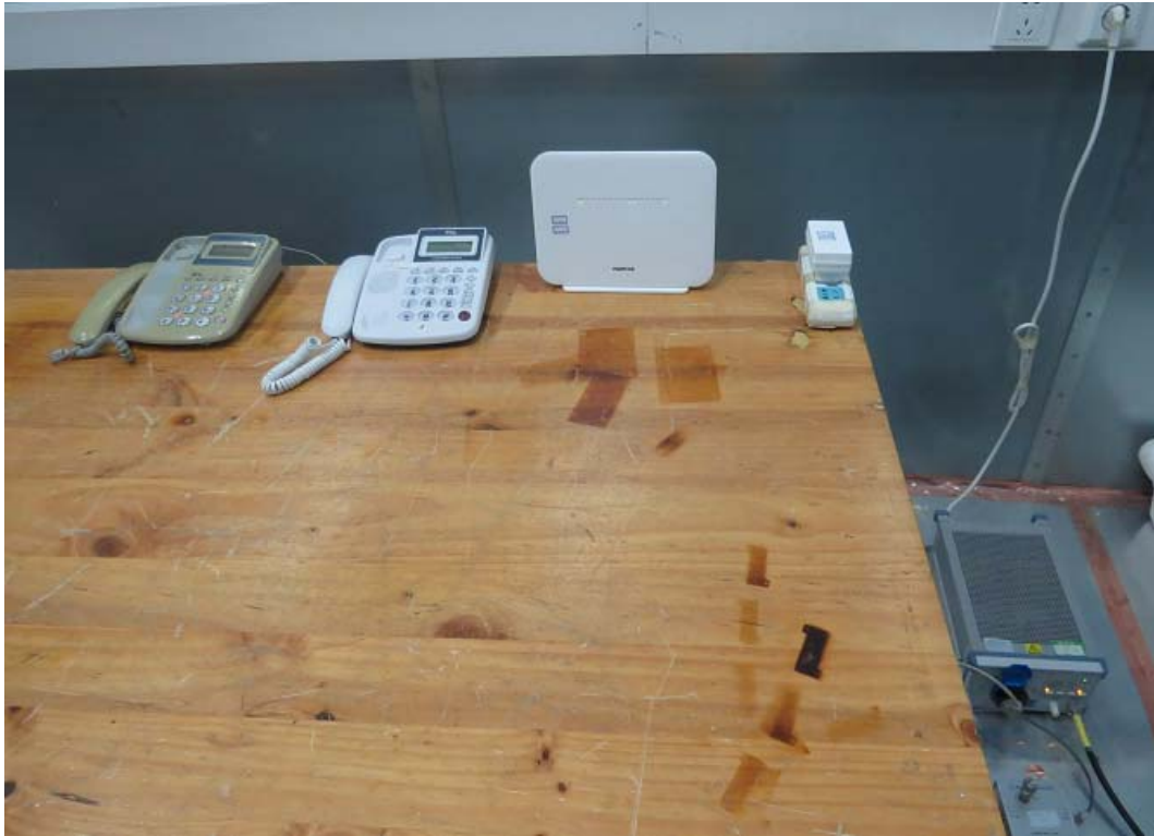
Picture 2 Conducted Emission Test Setup
