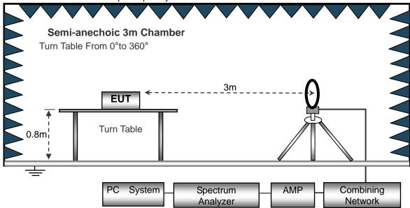
(B) Radiated Emission Test-Up Frequency 30MHz~1GHz
