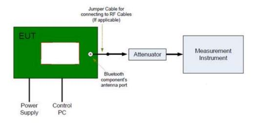
Setup diagram for radiated tests below 30MHz
