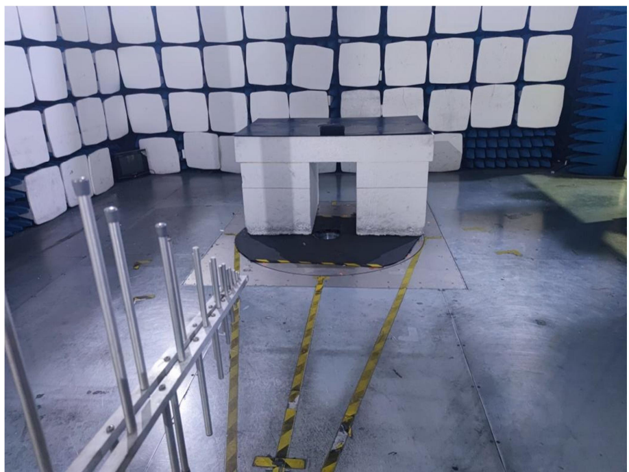
Radiation Emission Test Setup (30MHz to 1GHz)
