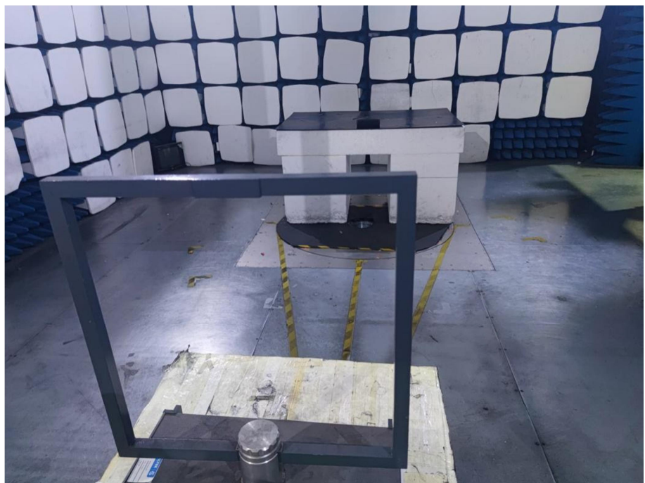
Radiation Emission Test Setup (Below 30MHz)
