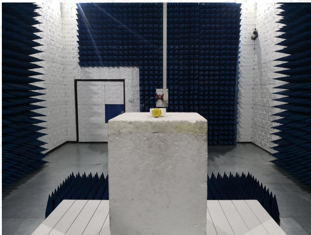
RADIATED EMISSION TEST SETUP ABOVE 1GHZ
