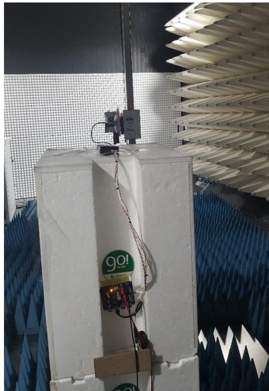
Figure B8. Radiated emission Test Setup High Range – Back side
