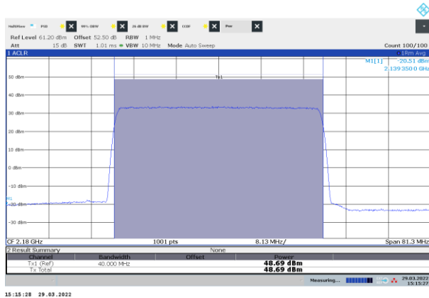
Figure 8.1-21: Power of NR 40 MHz channel bandwidth, single carrier operation, sample plot, top channel
