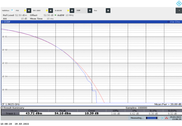
Figure 8.2-27: CCDF sample plot, NR 40 MHz channel bandwidth
