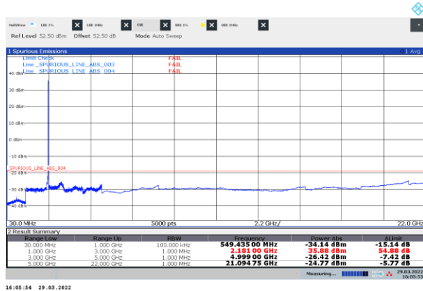
Figure 8.3-3: Conducted spurious emissions of NR 25 MHz top channel, single carrier operation
