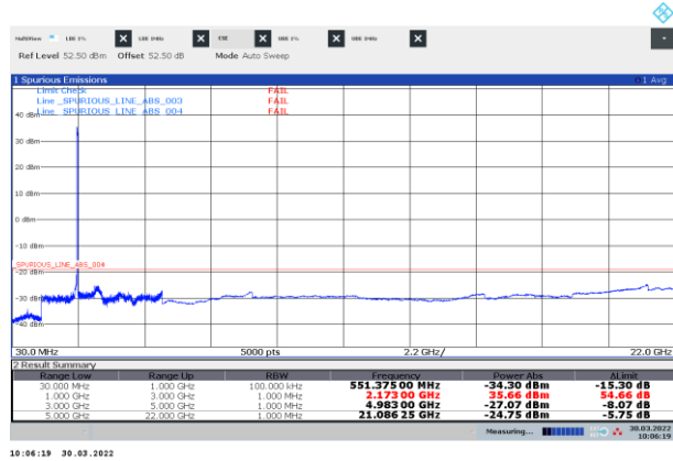
Figure 8.3-24: Conducted spurious emissions of multi-RAT operation, LTE 5 MHz + NR 25 MHz, top
