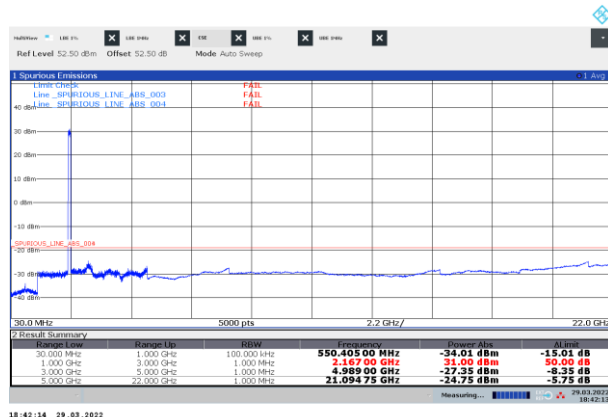
Figure 8.3-20: Conducted spurious emissions of NR 30 MHz three-carrier operation, top
