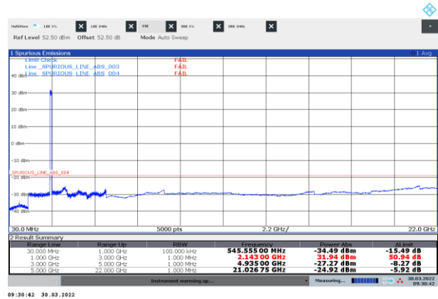
Figure 8.3-16: Conducted spurious emissions of NR 40 MHz two-carrier operation, top
