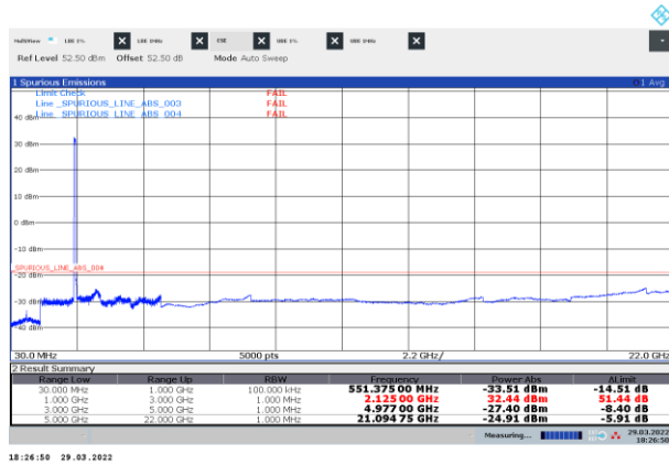
Figure 8.3-13: Conducted spurious emissions of NR 30 MHz two-carrier operation, bottom
