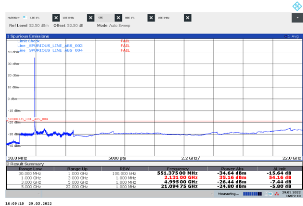
Figure 8.3-4: Conducted spurious emissions of NR 30 MHz bottom channel, single carrier operation
