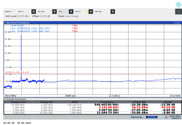
Figure 8.3-2: Conducted spurious emissions of NR 25 MHz mid channel, single carrier operation
