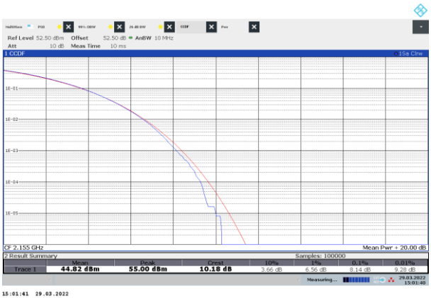
Figure 8.1-26: CCDF sample plot, NR 30 MHz channel bandwidth
