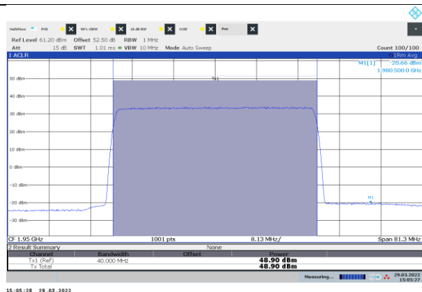
Figure 8.2-19: Power of NR 40 MHz channel bandwidth, single carrier operation, sample plot, bottom channel
