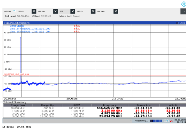
Figure 8.3-7: Conducted spurious emissions of NR 40 MHz bottom channel, single carrier operation
