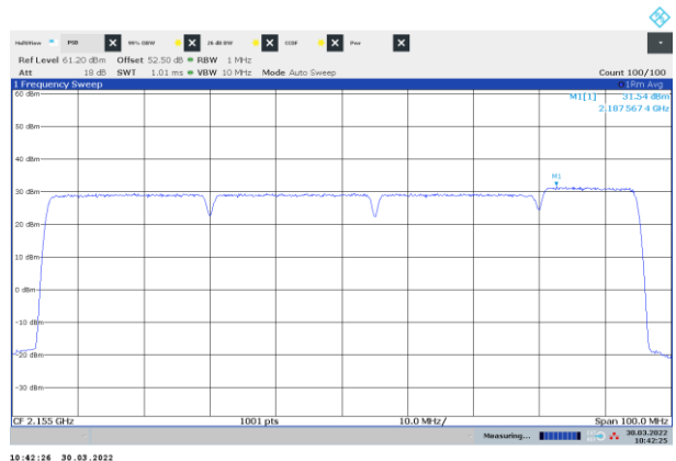
Figure 8.1-12: PSD of NR 25 MHz and 15 MHz channel bandwidth, four-carrier operation (3x 25 MHz + 1x15 MHz), sample plot, mid channel
