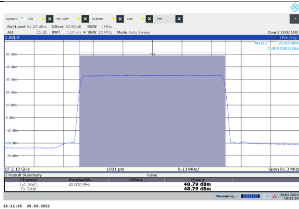
Figure 8.1-19: Power of NR 40 MHz channel bandwidth, single carrier operation, sample plot, bottom channel
