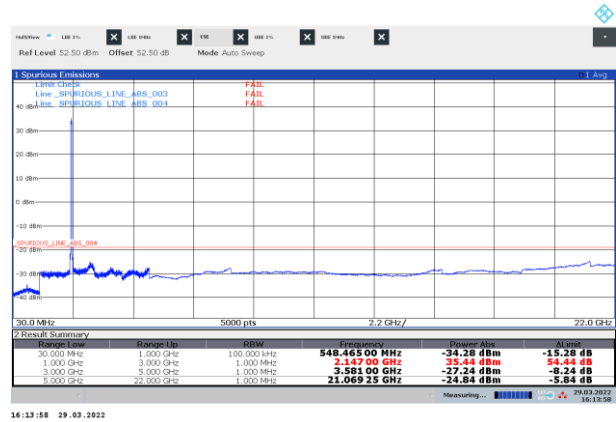
Figure 8.3-8: Conducted spurious emissions of NR 40 MHz mid channel, single carrier operation
