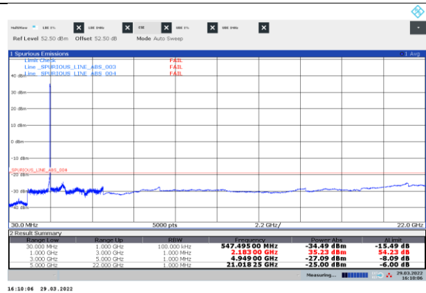
Figure 8.3-6: Conducted spurious emissions of NR 30 MHz top channel, single carrier operation
