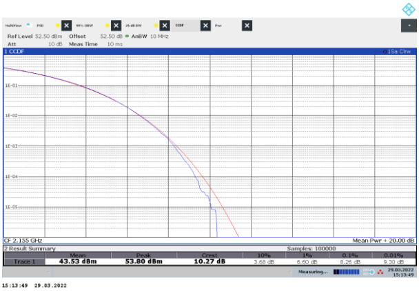
Figure 8.1-27: CCDF sample plot, NR 40 MHz channel bandwidth
