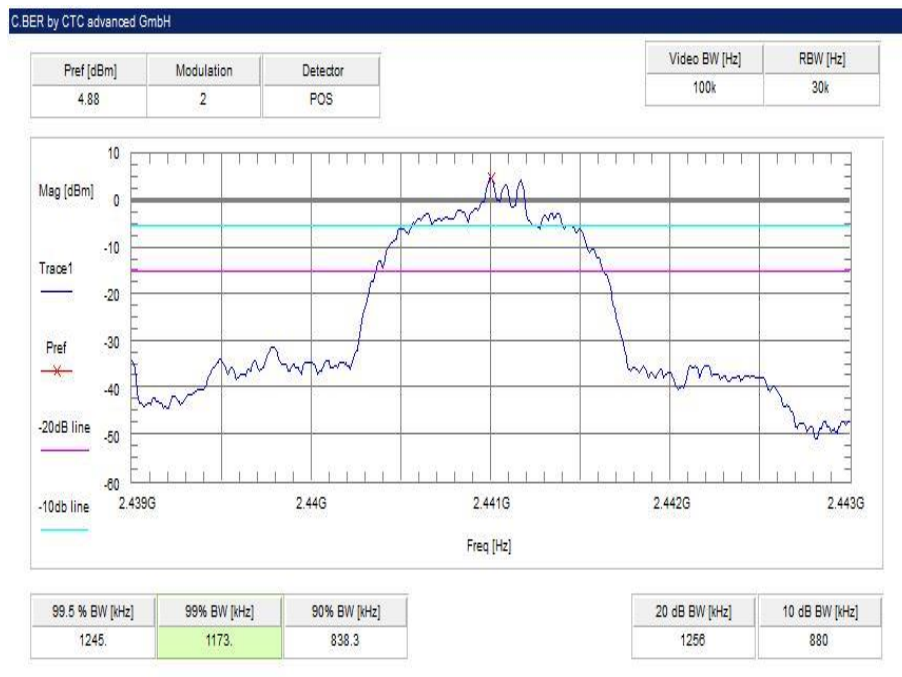
Plot 8: middle channel – 2441 MHz, 8 DPSK modulation
