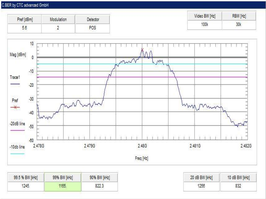
Plot 9: highest channel – 2480 MHz, 8 DPSK modulation
