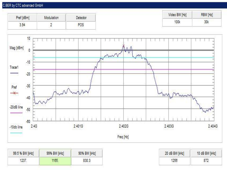
Plot 7: lowest channel – 2402 MHz, 8 DPSK modulation
