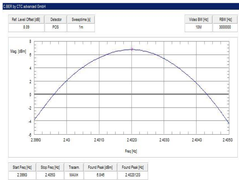
Plot 7: lowest channel – 2402 MHz, 8 DPSK modulation
