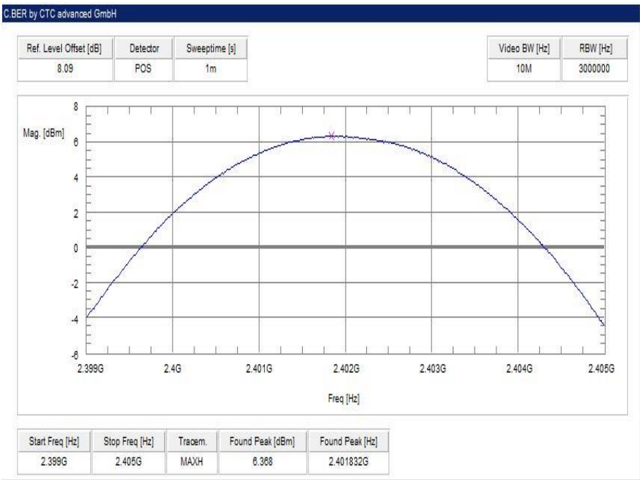
Plot 4: lowest channel – 2402 MHz, Pi / DQPSK modulation
