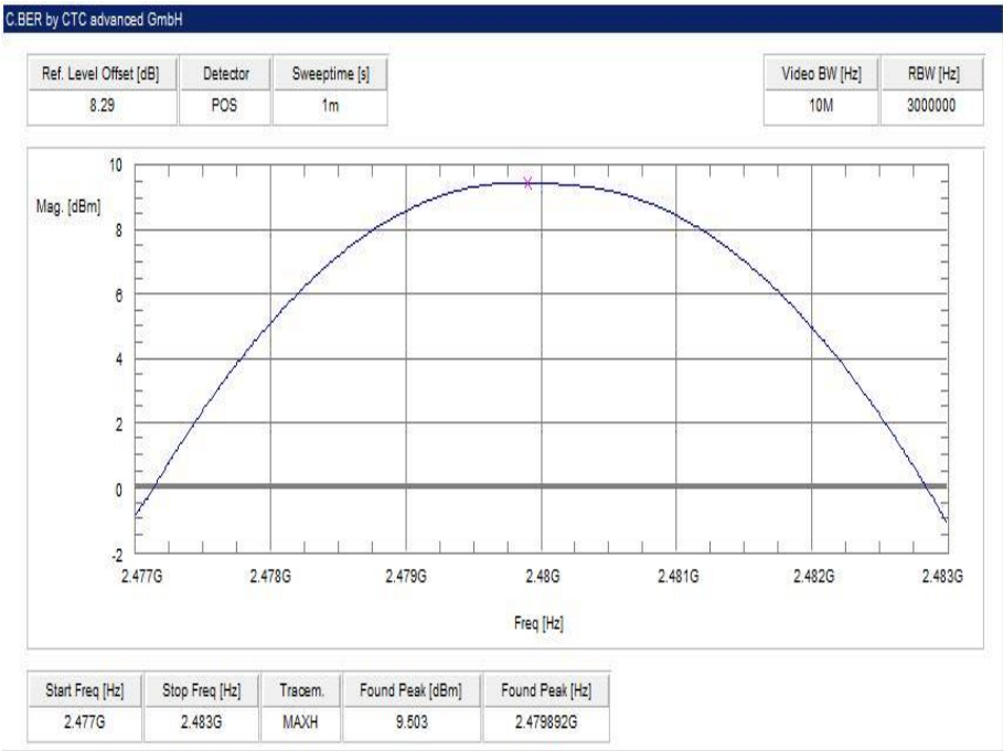
Plot 3: highest channel – 2480 MHz, GFSK modulation
