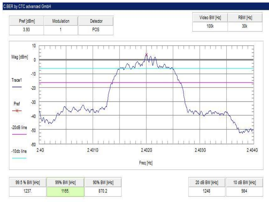
Plot 4: lowest channel – 2402 MHz, Pi / DQPSK modulation
