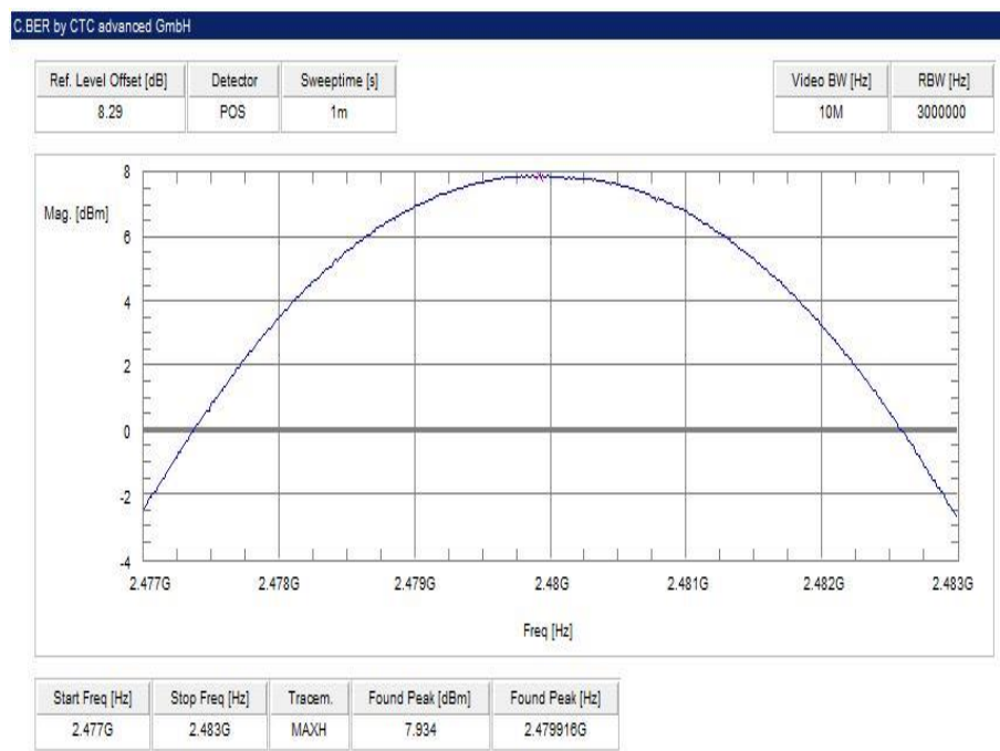
Plot 6: highest channel – 2480 MHz, Pi / DQPSK modulation
