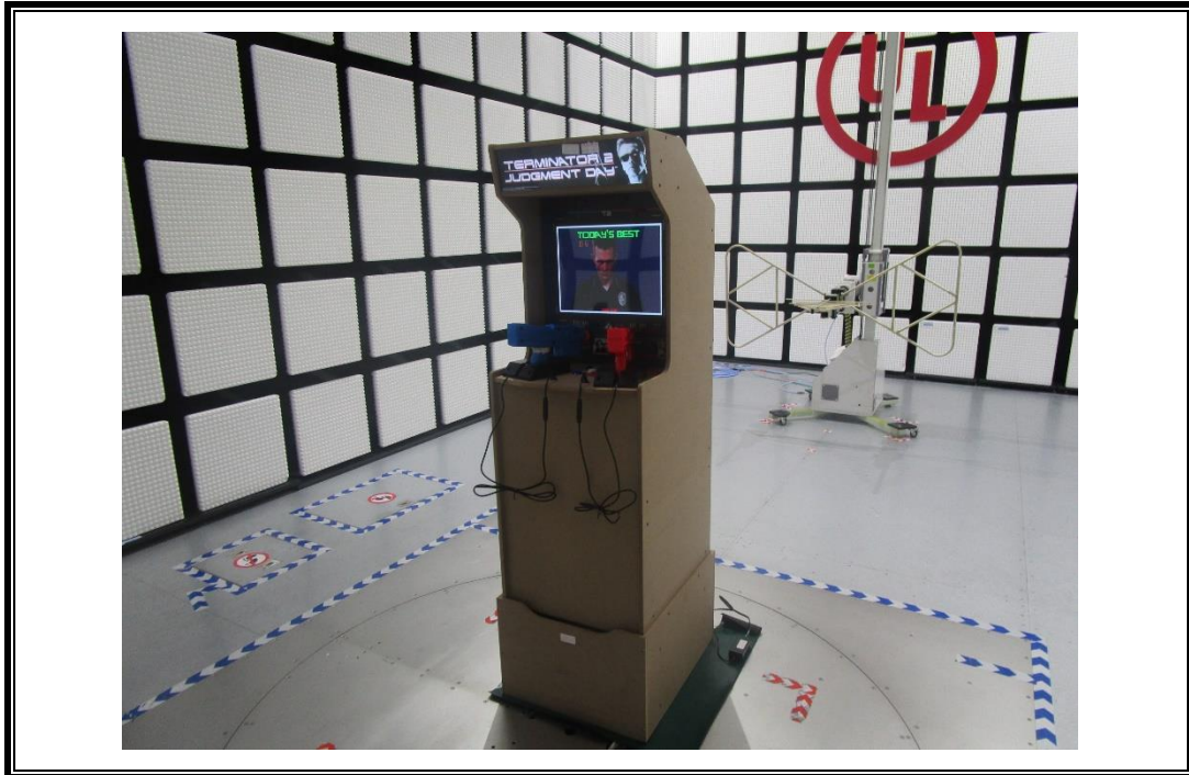
RADIATED RF MEASUREMENT SETUP (30MHz ~ 1 GHz)
