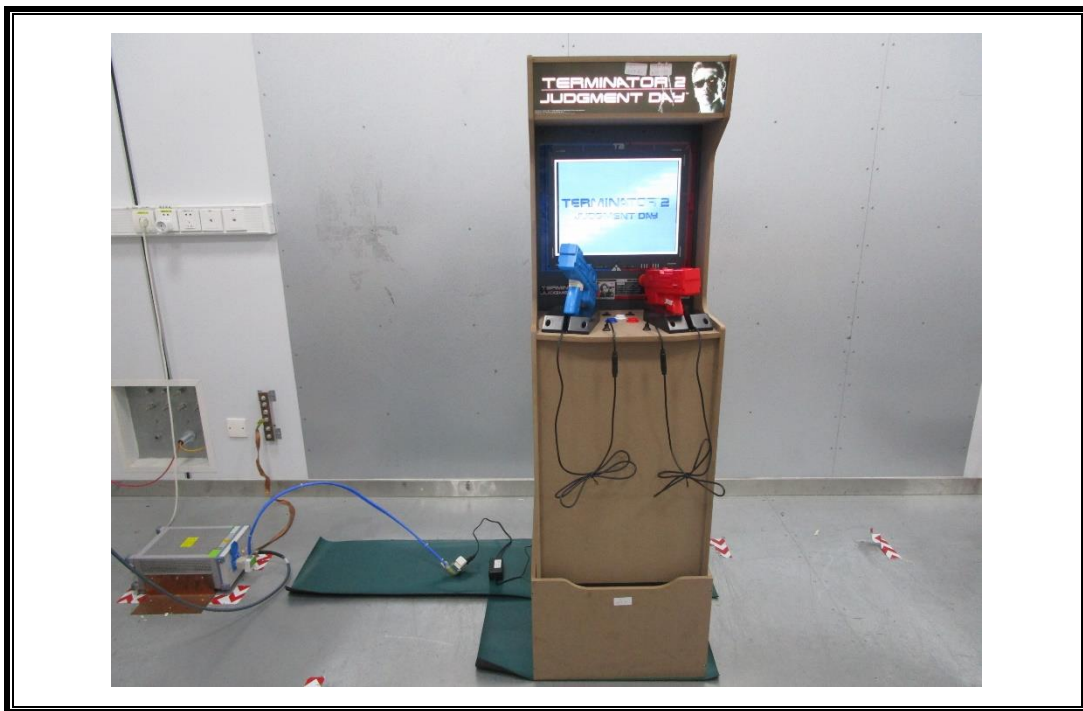
AC POWER LINE CONDUCTED EMISSIONS
